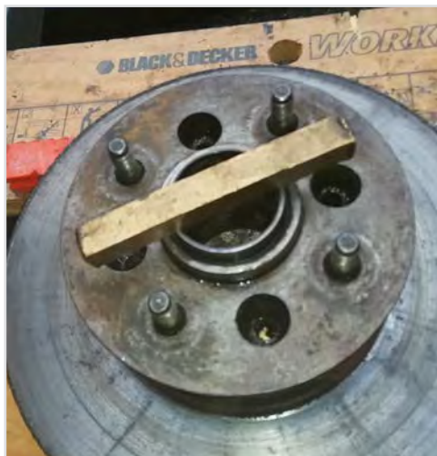
Drifting in the new bearing races using a brass drift
