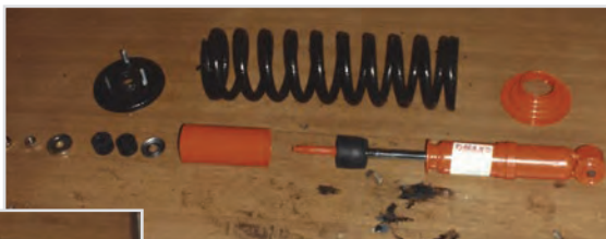
New Shock Absorber and Spring Assembly parts ready for re-assembly
