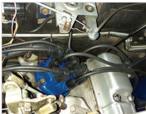
Photo 3: Clean distributor cap with new leads
