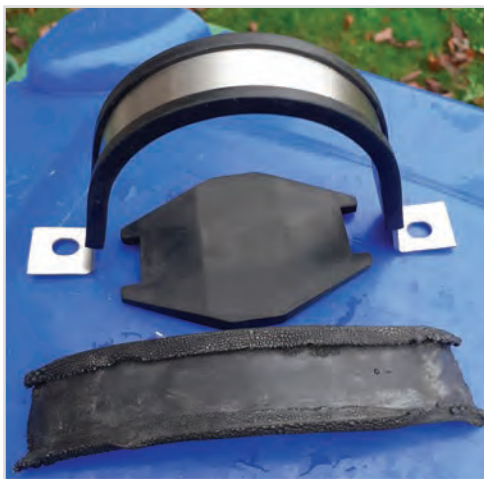
Photo 5: Old wiper motor strap rubber with new strap, rubber and cushion pad
