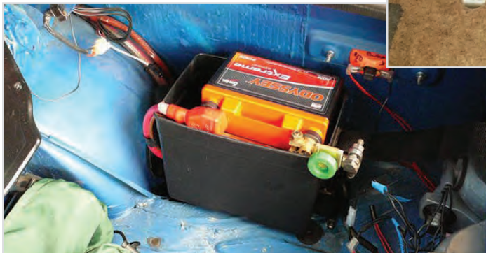
TR8 Battery Boot Conversion
