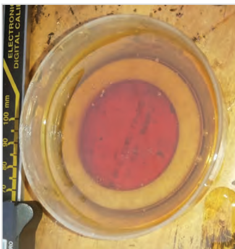
Soaking a new Seal in Oil before fitting
