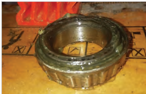
Grease the roller bearings generously with a good quality grease.
