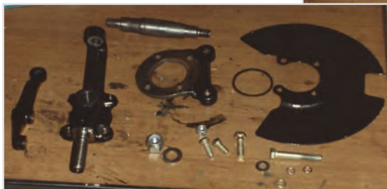
Vertical Link Assembly parts painted ready for re-assembly
