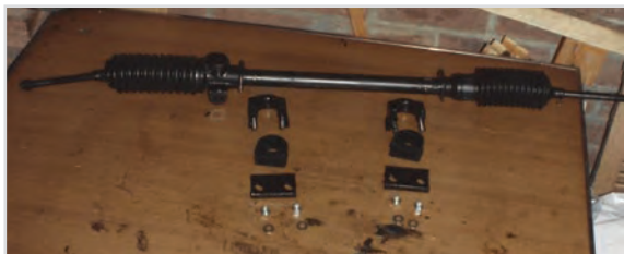
Re-conditioned Steering Rack and mountings painted with new bushes and u bolts.
