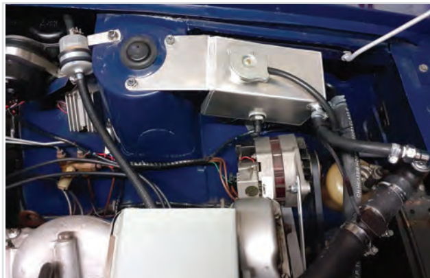
Photo 2: Stagweber tank and Tony Hart alternator bracketry.
