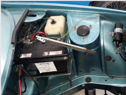
TR7 Battery Location Under Bonnet
